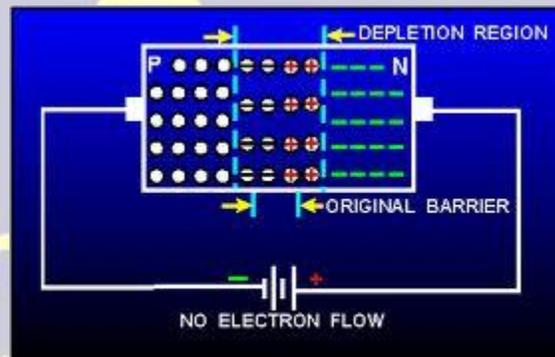
When a P-N junction is joined with a battery in such a way that its P-type is connected to negative terminal and N-type is connected with positive terminal then a reverse potential creates an electric field which acts in the direction of field of Potential resistance. Therefore, a powerful field produces on the junction. And height of resistance raises. The high of resistance resists against the flow of electrons. Hence, no current flows. This whole process is known as Reverse Biased.
