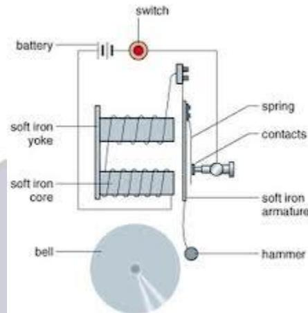
It is an electromagnetic instrument used to produce sound.
