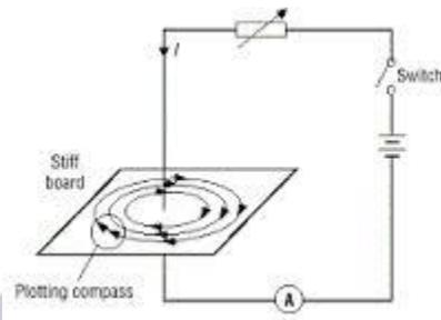
When current passes through any conductor it becomes magnet and a magnetic field develops around it. The strength of magnetic field is directly proportional to the amount of current flowing through the galvanometer and inversely proportional to the distance around it.
