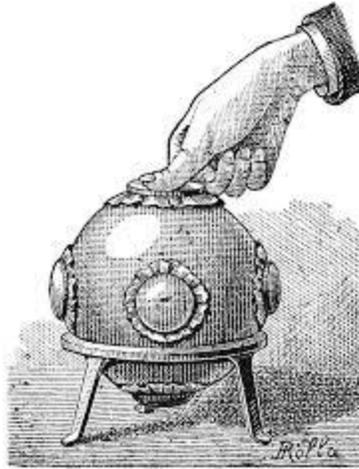
According to this principle, if a pressure is applied to a liquid contained in a vessel, it is transmitted pressure equally in all direction and acts perpendicularly to the walls of the container. This was discovered by Blaise Pascal, and is known as Pascal's Principle.
