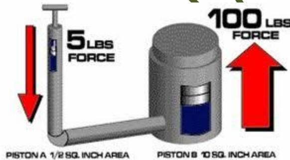
The working of hydraulic press is same hydraulic lift, in a hydraulic press the piston 'B' is used to compress any material over it a rigid roof material is placed between roof and piston 'B'. When force is applied on piston 'n' then B moves upwards. It compresses cotton into a compact bale.
