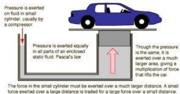
It is filled with some incompressible fluid. By pressing cylinder 'A', the pressure is transmitted equally according to Pascal's principle to the piston of the cylinder 'B' and B moves upward. The piston 'B' is used as a platform for a car or any heavier object to be lifted.
