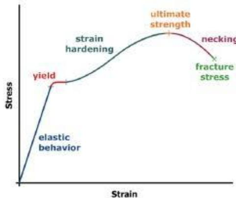
In this graph, if we increase stress then strain will also increase. Even a body reaches to a point "x", here elasticity maintained. If stress kept continues then the body will go to Plastic region. It means elasticity
