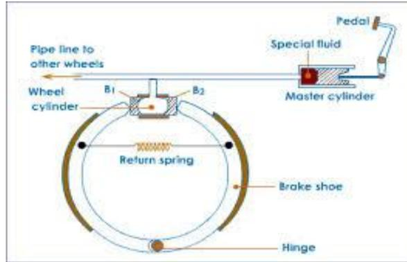
System is used in vehicle, consists of a master cylinder joined by tubes to four smaller cylinder, one for each wheel of vehicle. The master cylinder and each of the brake cylinders are provided oil tight pistons. When we push on the brake pedal it causes a force on the piston in the master cylinder. This pressure transmits equally in all directions.
