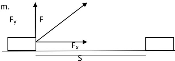
In the above figure. Force “F” divided into two components vertical  $F_y$  and horizontal  $F_x$ .  $\theta$  is the angle between them. So the dot product of  $F_x$  and displacement “S” is given by:
