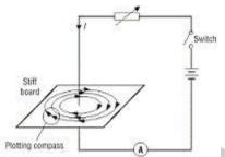
When current passes through any conductor it becomes magnet and a magnetic field develops around it. The strength of magnetic field is directly proportional to the amount of current flowing through the galvanometer and inversely proportional to the distance around it.
