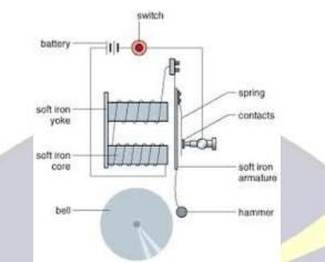
It is an electromagnetic instrument used to produce sound. Construction:
