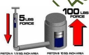
The working of hydraulic press is same hydraulic lift, in a hydraulic press the piston 'B' is used to compress any material over it a rigid roof material is placed between roof and piston 'B'. When force is applied on piston 'n' then Bymoves upwards. It compresses cotton into a compact bale.
